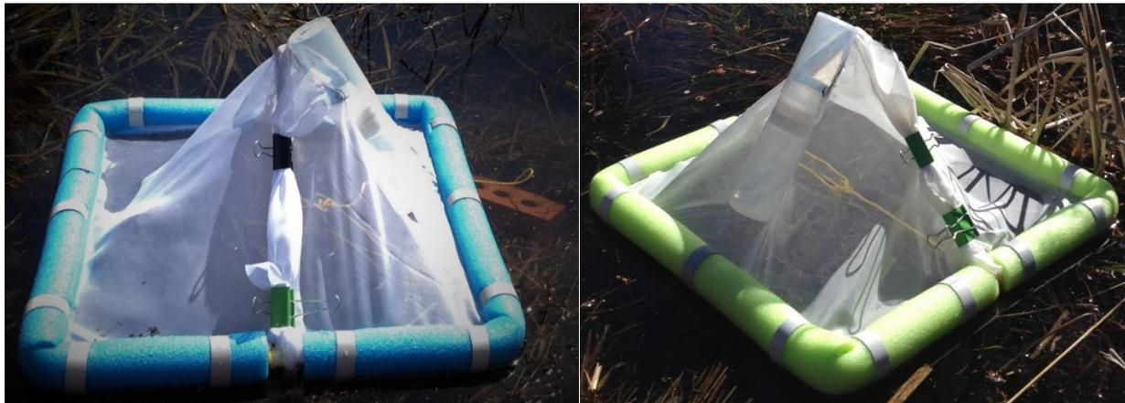
*Figure 2* Emergence trap design is framed with a pvc-skeleton, draped with fine transparent netting that directs emergent insects into the collection cup opening at the top of the frame. Polyethylene foam allows the trap to float while tethered by an adjustable rope and anchored by a brick.
